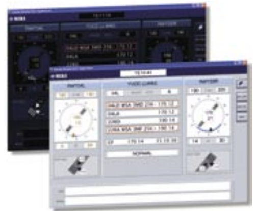
For each touchdown zone, the Vaisala AviMet® LLWAS alert screen displays the threshold windshear alerts and wind speed and direction. It also displays the center field wind speed and direction and system status.
