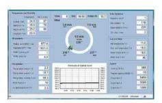
Vaisala MCC301software displays and logs data from AWS310 weather station. It is easy to install and operate. The data distribution feature allows several client PCs to gather weather data from the master PC.
