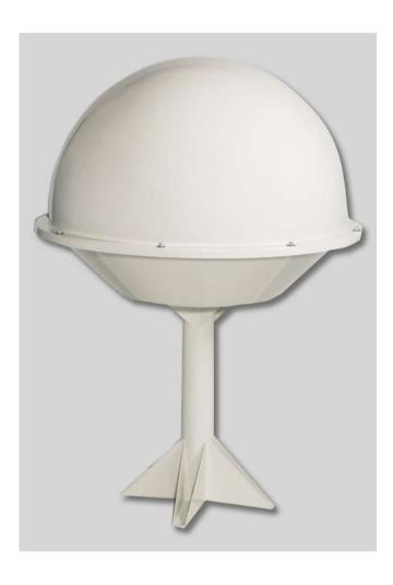
The Vaisala Telemetry Antenna RB31 has no moving parts and is controlled automatically by a Vaisala telemetry receiver. The RB31 is delivered as a complete unit and is easy to install. The RB31 is protected by a radome against rain and high winds, and has six monopoles with corner reflectors and a cross dipole. The dipole
