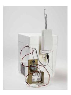
pump base. The heating is powered by an additional battery with a voltage range from 9 to 19 V. The recommended battery is a 9 V square battery that can easily be fitted onto the ozone sensor frame inside the ozone box.
