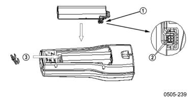
Figure 19 Installing the Battery Pack
