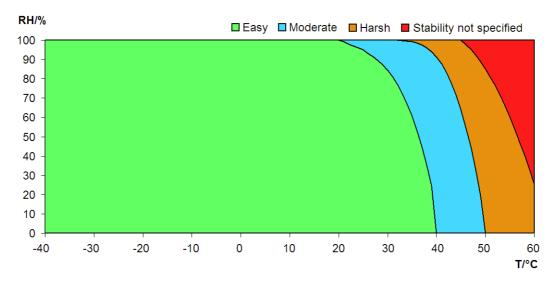
Figure 11 GMP343 Operating Conditions
