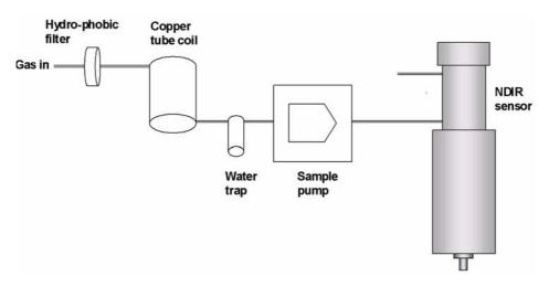
Figure 3 Components of the Sampling System
