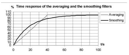
Figure 9 The Difference of the Two Filters in Time Response
