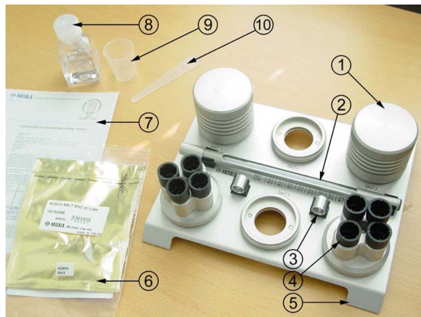
Figure 1 The HMK15 calibrator with some accessories (*)
