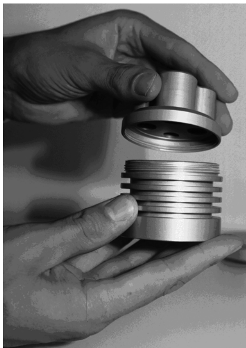
Figure 5 Close the chamber with the chamber cover
