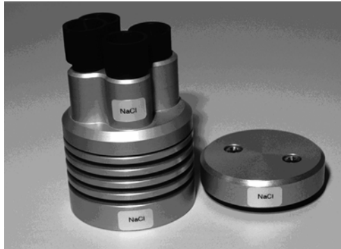
Figure 6 Mark the chamber and covers with stickers
