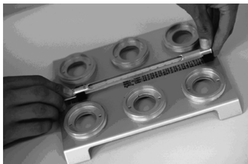
Figure 10 Place the thermometer in holders when not in use
