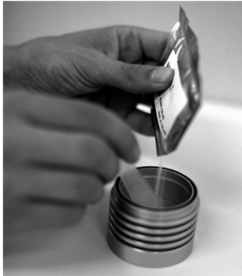
Figure 4 Sprinkle a correct dose of salt into the chamber stirring constantly
