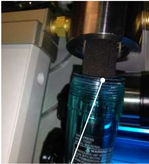
Step 2 : Check the O-ring seal. DO NOT lose it !!! Replacement O-ring seal P/N : SC024-55
