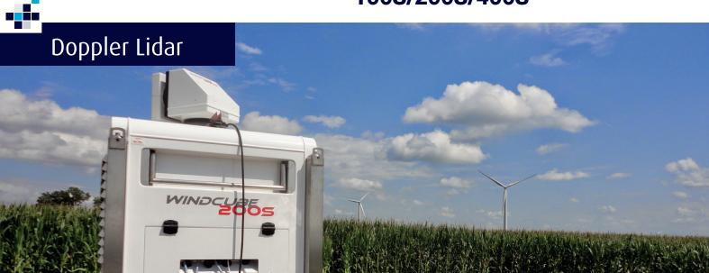
Scanning wind doppler Lidars systems offer a fully integrated operational capacity to improve wind measurement at any stage of a wind farm project, from prospecting to operation. WINDCUBE 100S / 200S / 400S perform a full 3D mapping of the atmosphere to provide enhanced measurements of wind speed and direction.
