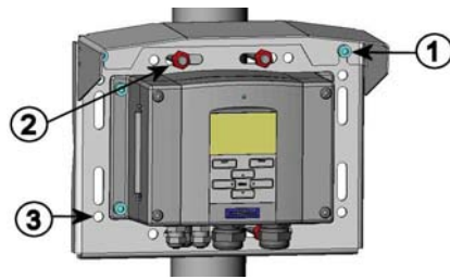
Figure 13 Mounting Rain Shield with Installation Kit
