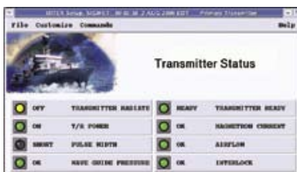
Fault messages from BITE (BITE examiner utility) are displayed with audio beep or voice synthesis alert.
