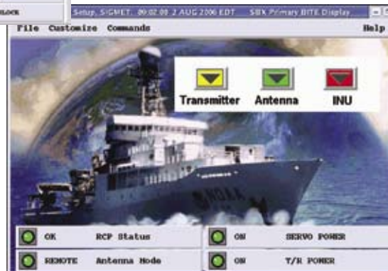
Fault messages from BITE (BITE examiner utility) are displayed with audio beep or voice synthesis alert.
