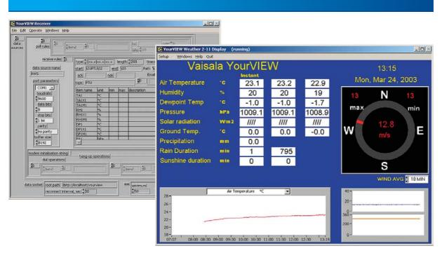
Vaisala Real-time Display Software YourView is graphical user interface software for Vaisala automatic weather stations. It offers a graphical presentation of real-time and logged data and allows you to log data to your PC hard disk.
