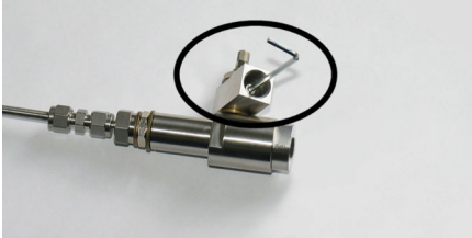
Figure 18 Removing the leak screw
