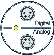
Figure 8 DMT143 digital and analog connectors
