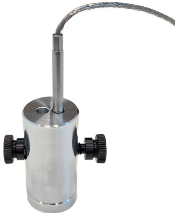
Figure 9 Thermal dampener block with TMP115 probe head inserted
