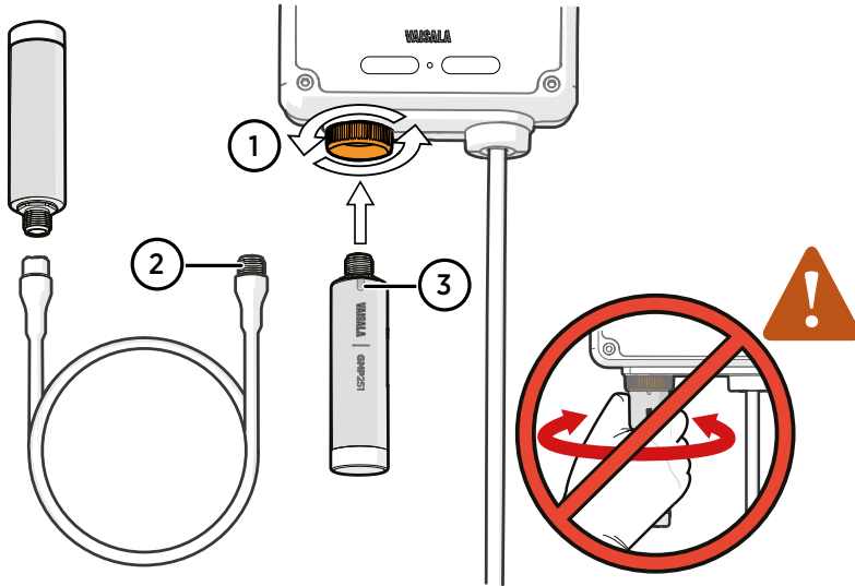
Figure 11 Connecting probes and cables to Indigo200
